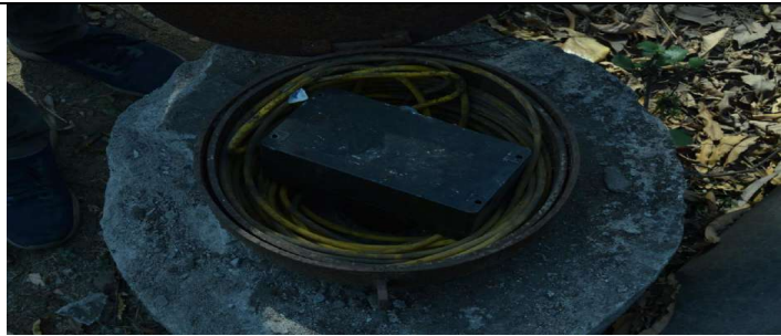
Piezometric with Automatic Well Recorder At Sodepur Colliery
